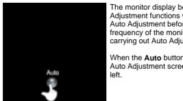
The monitor display becomes more stabilized if adjusted by Auto Adjustment functions when the monitor is installed for the first time. Try Auto Adjustment before attempting Manual Adjustment. Ensure the clock frequency of the monitor matches that of the computer video card before carrying out Auto Adjustment.
